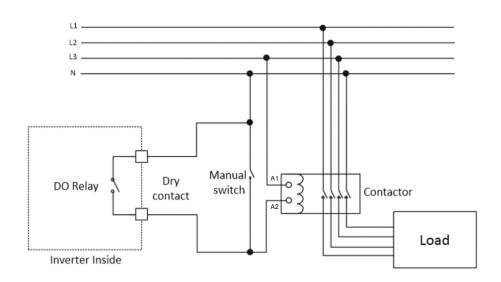
The inverter integrates a Dry contact which can be connected to the contactor to control the loads on or off. If DO relay is off at inverter side, A1 and A2 of the contactor will connect to L and N, so that the contactor will be turned off. Then the load will connect to grid or inverter backup output port through the contactor.
