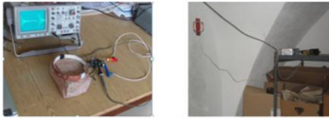
Fig. 3. The tested device and its placement in the cellar.
