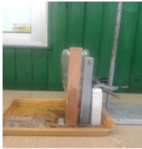
Fig. 4. Water intake test.
